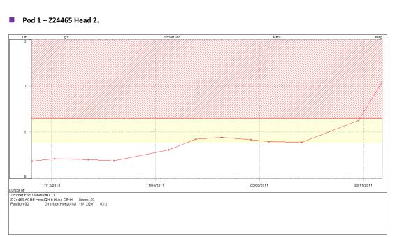
Motor DE Bearing – Readings obtained have increased considerably since Nov. reading.
