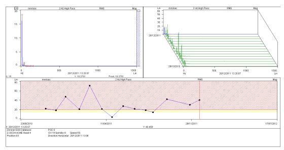
**Spindle Balance** – Readings obtained from the spindle bearing have shown a significant increase in mm/s velocity vibration at 15Hz. This activity is indicative of imbalance.
