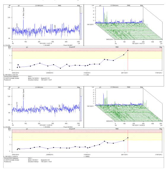
**Motor Bearings** – Readings obtained from the motor bearings have shown a progressive increase in g's acceleration activity on this visit. Evidence of increased overall noise levels is evident particularly at the motor NDE.
