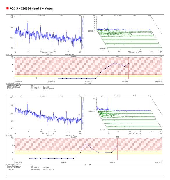
**Motor Bearings** – Readings obtained from the motor bearings have shown a further increase in g's acceleration activity on this visit, both overall noise levels and impacting energy at frequencies possibly related to the bearings. Bearing numbers would be required to confirm this.
