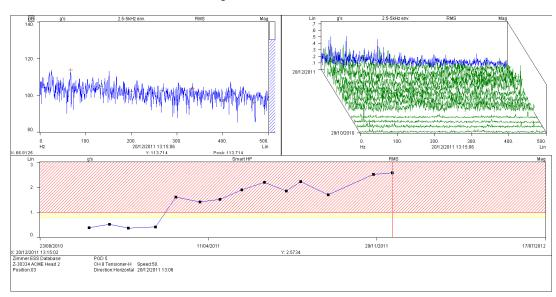
**Tensioner Bearing** – Readings obtained from the tensioner bearings have shown a progressive increase in g's acceleration activity, overall noise levels are raising but no impact energy is evident at this time.
