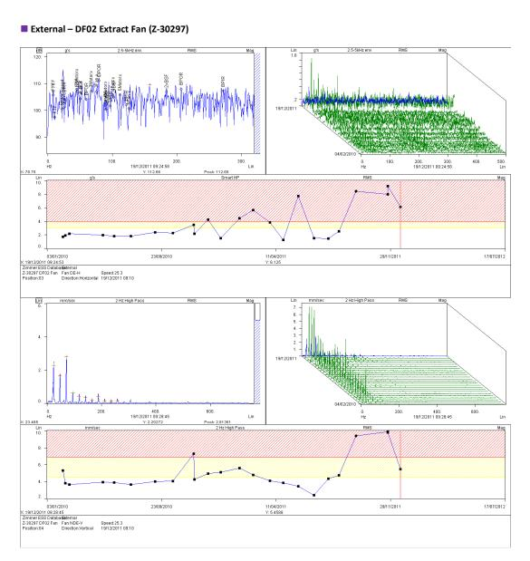
**Imbalance** – Readings obtained throughout the unit have shown a reduction of the mm/s velocity vibration at the fan shaft rotational frequency on this visit.
