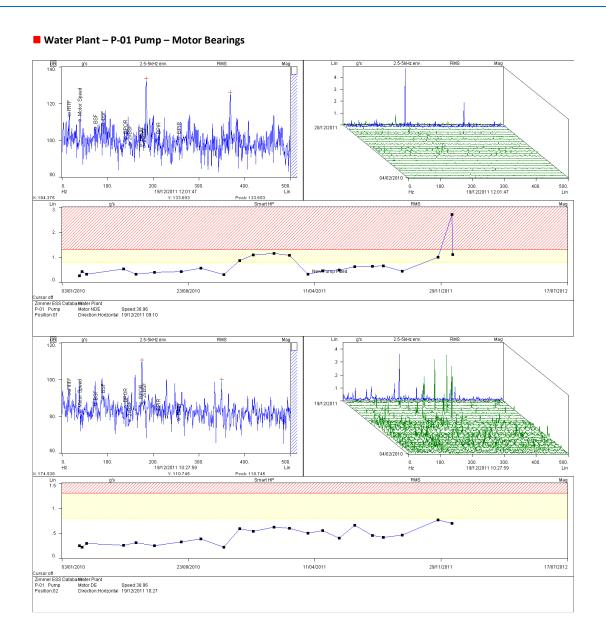
**Motor Bearings** – Readings obtained from the motor bearings have shown a significant increase in g's acceleration activity on this visit. Evidence of increased overall noise levels is evident at two running speeds and the bearing data displays impact energy.
